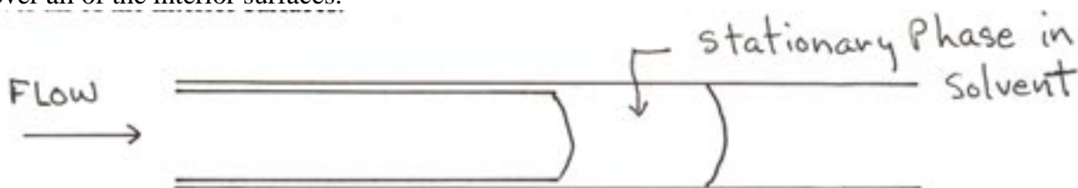
Moving plug technique for coating a capillary column
