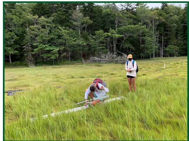
Photo credit: Bev Johnson. Measuring the pin heights for SET 4 using the sediment elevation table on 08/27/2020.
