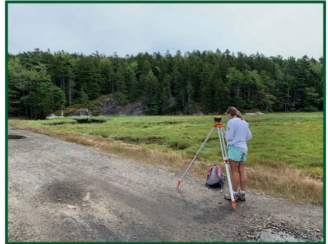
Photo credit: Bev Johnson. Using the tripod, on the causeway, and auto-level to measure the stadia rod measurements for SET 4 on 08/27/2020.
