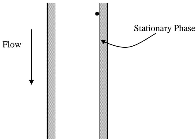
**The dot represents a molecule that has just left the stationary phase is about to diffuse across the mobile phase and re-encounter the stationary phase on the other side of the column.**
