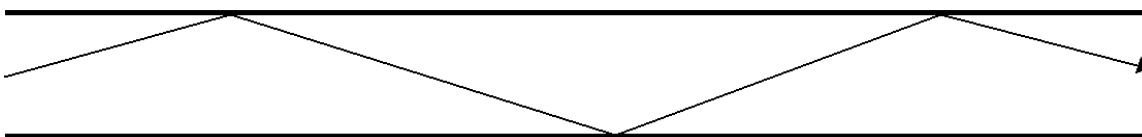
Figure 35. Complete internal reflection of a light beam inside a fiber optic.
